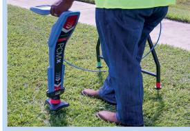
One second mapping measurements combined with simultaneous ACCA and ACVG data gathering makes surveying faster.
